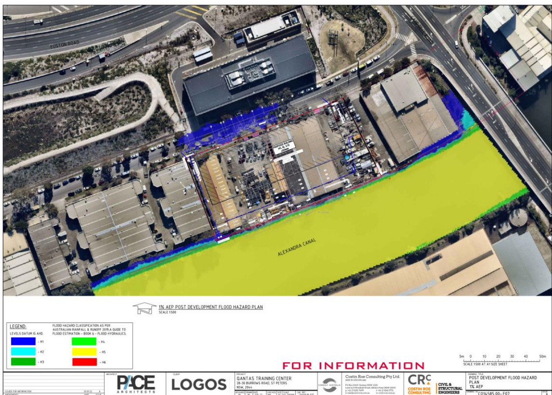
Figure 7.18: 1% AEP Post-developed Flood Hazard Categorisation
