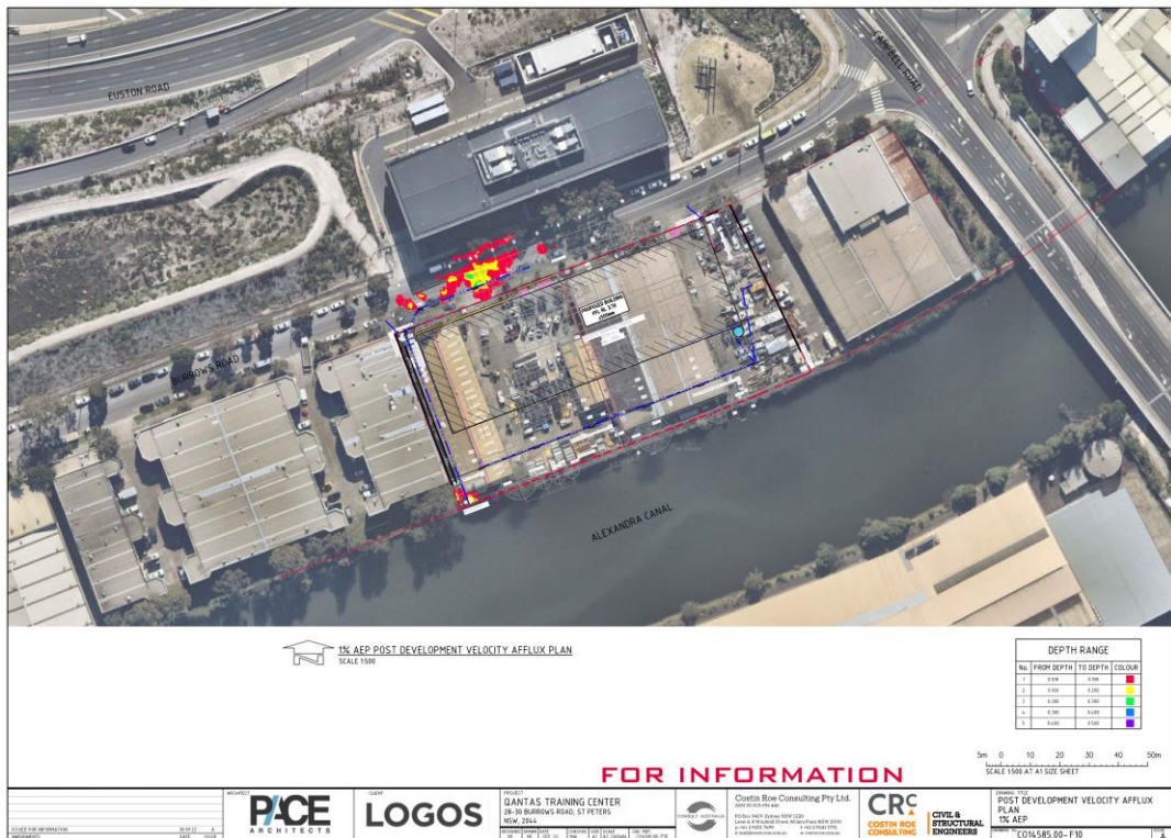
Figure 7.20: 1% AEP Post Developed Flood Velocity Afflux
