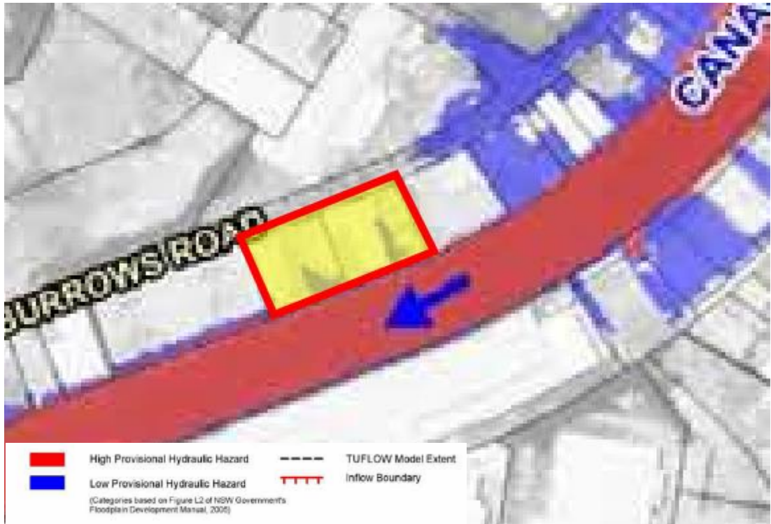
Figure 7.9. M5 EIS - 1% AEP Provisional Flood Hazard
