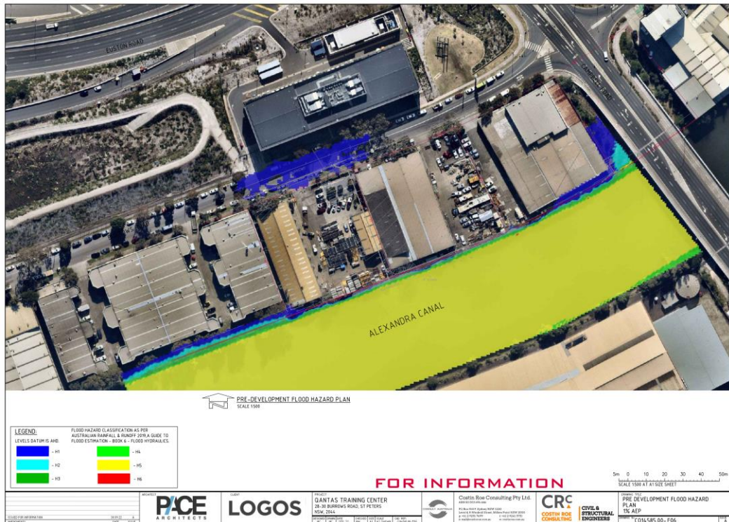
Figure 7.15: 1% AEP Pre-developed Flood Hazard Categorisation
