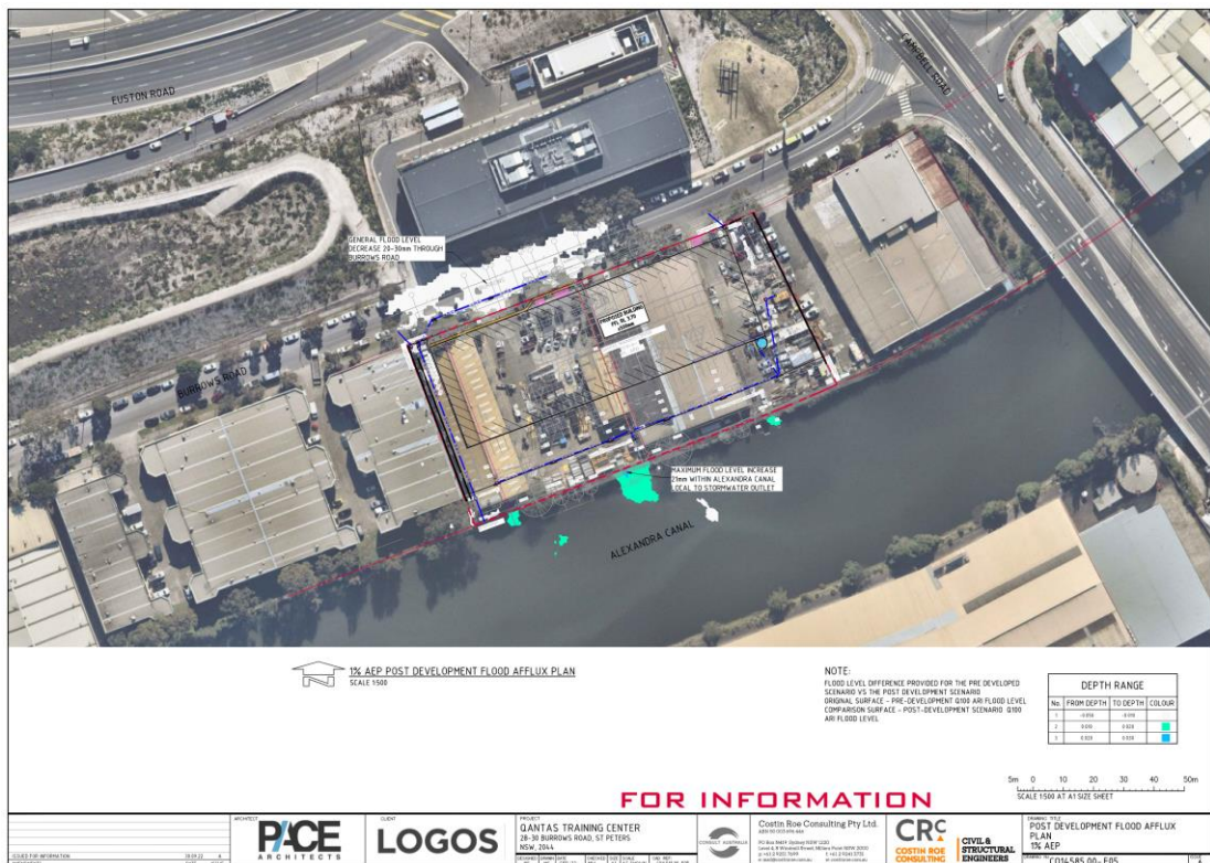
Figure 7.19: 1% AEP Post Developed Flood Level Afflux
