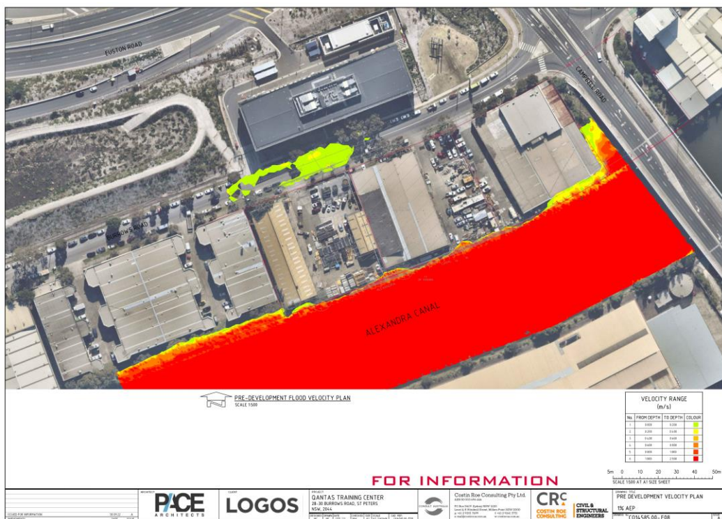
Figure 7.14: 1% AEP Pre-developed Velocity
