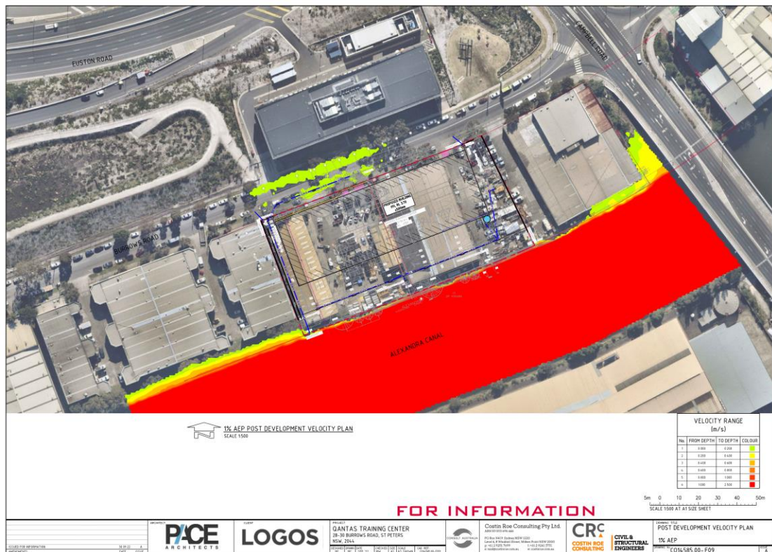
Figure 7.17: 1% AEP Post-developed Velocity
