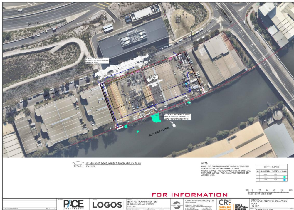
Figure E4.3: 1% AEP Flood Afflux Plan
