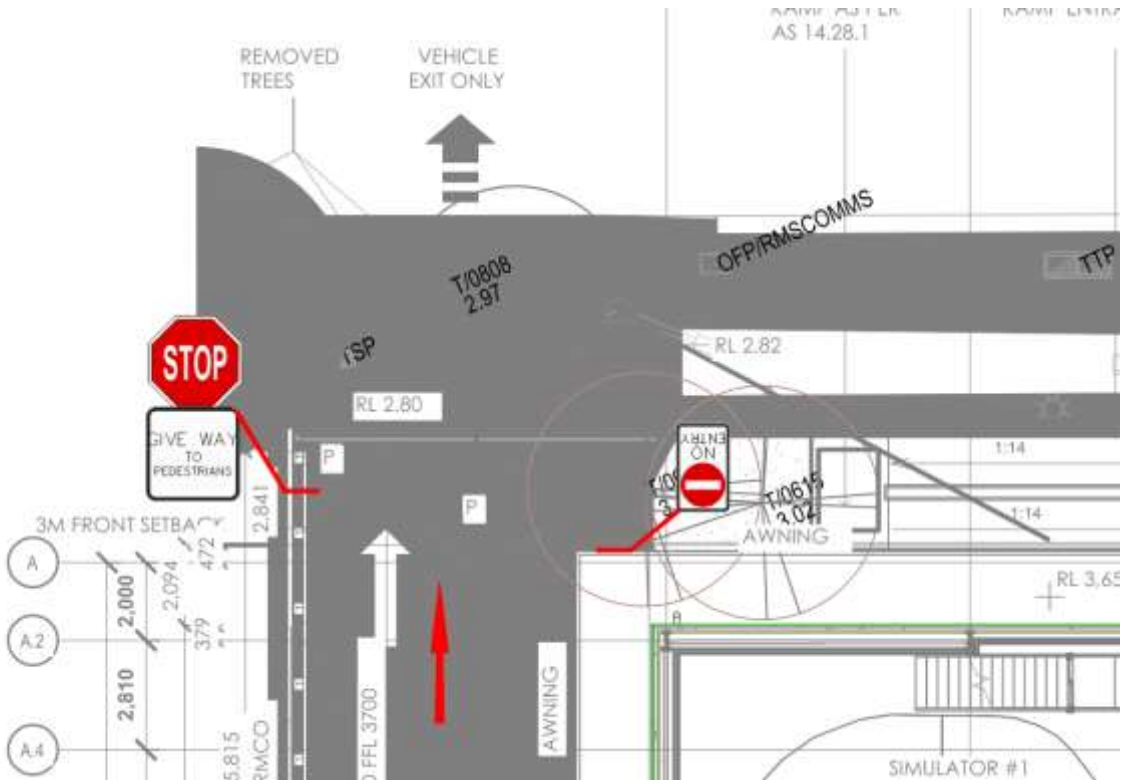
Figure 4: Exit Driveway Signage
